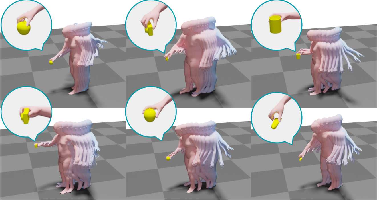
Figure 6. Representative motions generated by GOAL (GNet and MNet) for several object shapes, locations, body shapes and “start” poses.
